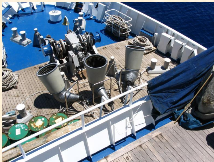
Fig.5 Antennas of the high-frequency SODAR system
