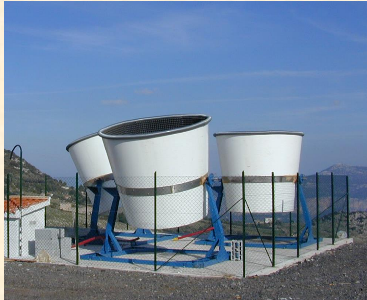
Fig.4 Antennas of the low-frequency SODAR system
